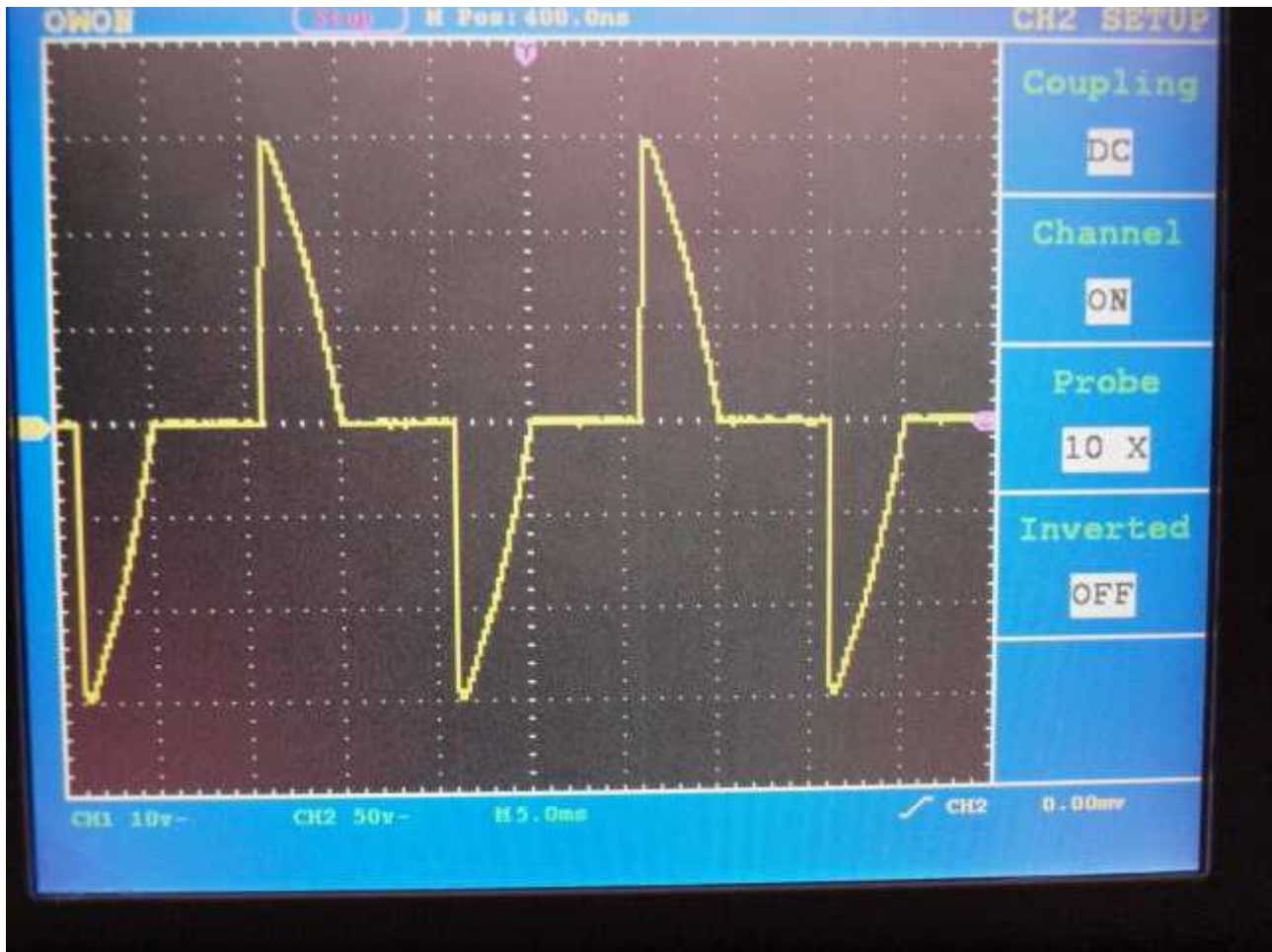
Pic 3; waveform with dimmer control and a 25ohm load (~4 Amps)
