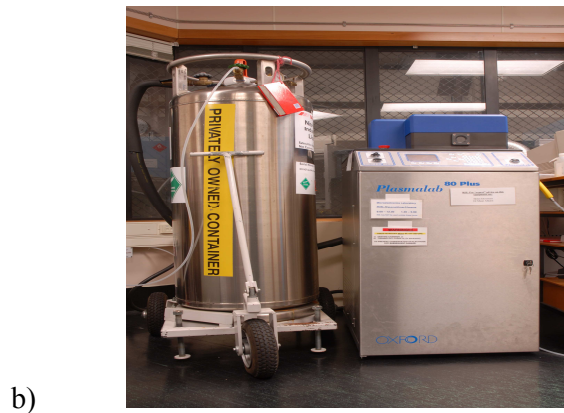
Figure 3-6 (a) A schematic of typical parallel plate reactive ion etching system, and (b) Oxford Plasma Lab 80 Plus system used in this study.
