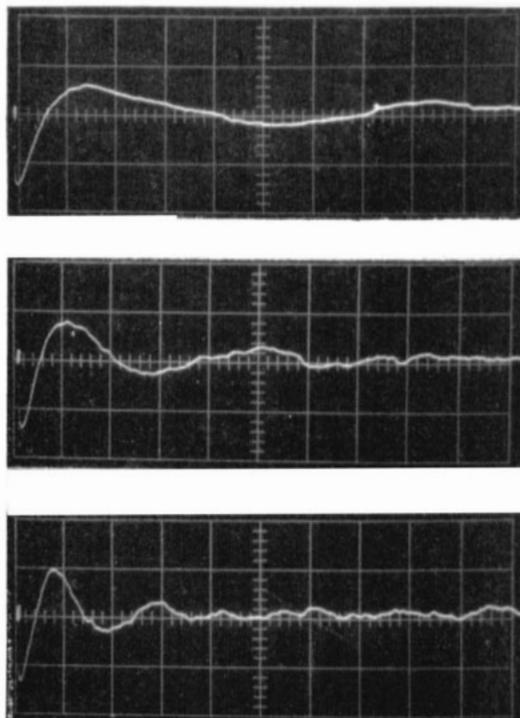
Figure 1. Oscillograms of  $\alpha$ -particle pulses from  $^{10}\text{B}(n, \alpha)^7\text{Li}$  at the anode of a corona-proportional counter at various corona currents (upper  $1 \mu\text{A}$ , middle  $5 \mu\text{A}$ , lower  $10 \mu\text{A}$ ). Time scale  $50 \mu\text{sec cm}^{-1}$ , amplitude sensitivity  $15 \text{mv cm}^{-1}$ . Pulses have been RC clipped at  $5 \mu\text{sec}$  time constant.
