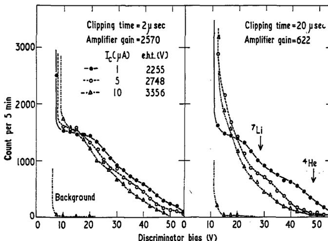
Figure 2. Neutron count rate against pulse-height discriminator bias at various corona currents. RC clipping of counter pulses at short time constant improves the stability of the count-bias plateau with changing corona current.
