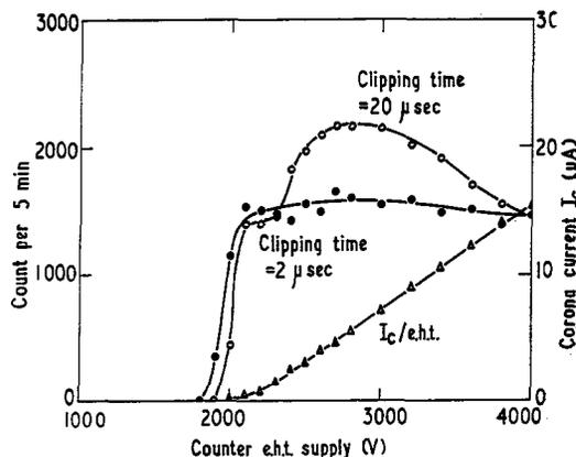
Figure 3. Variation of neutron count rate and corona current with counter e.h.t. supply voltage. Discriminator bias set at 15 v (see figure 2).
