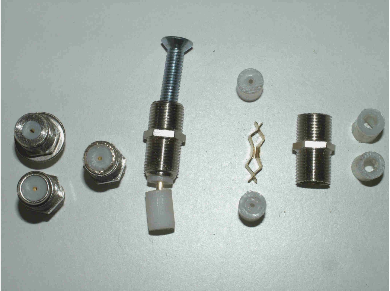
Diagram 1: Left to right in the above picture; regular F-female to female parts, file off the peened end as far as the insulator, pressing out the parts, pressed parts (2xHDPE insulators + contacts), file both ends away, drill out slightly smaller than the insulator on the coax.
