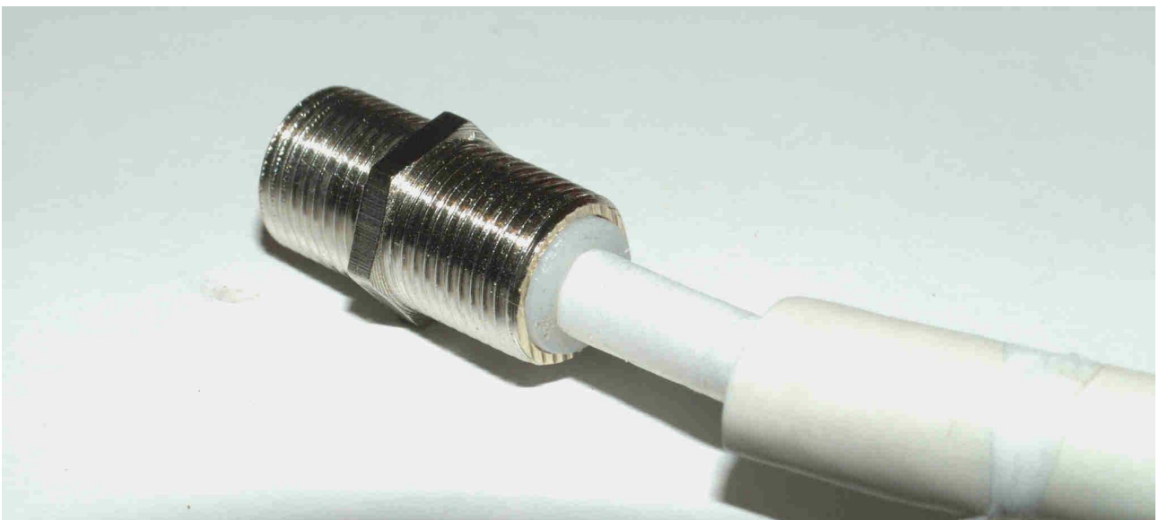
Diagram 5: insulator inserts into female insulator, the foamed PE seals up around the hole leaving no exposed centre conductor (F-screw outer not show). A similar connection took 5 kV for ten minutes and 15kV for a minute without any indication of insulator breakdown.
