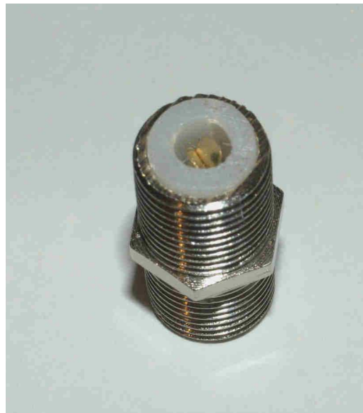
Diagram 3: finished 'HV' F-type f-f connector.
